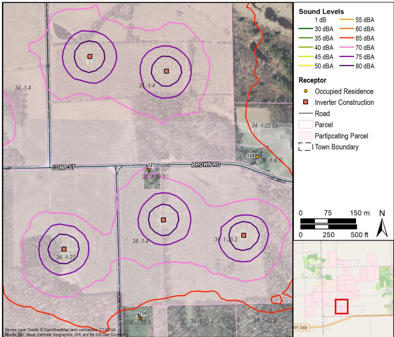
FIGURE 31: INVERTER CONSTRUCTION MODEL RESULTS, WORST-CASE RECEPTOR 127
