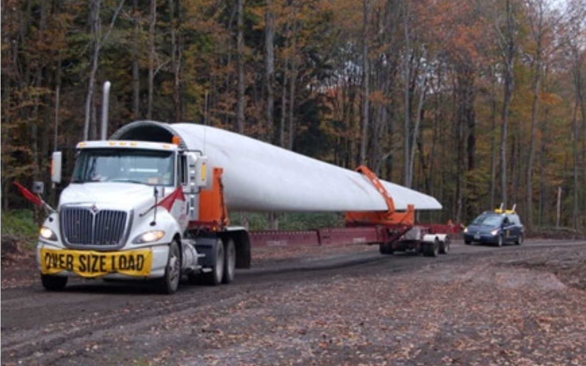
Figure 5.2-4. Transportation of Wind Turbine Components
